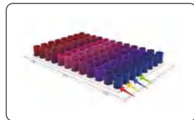
Unique side scan technology, all channels can be detected simultaneously, complete the scan of all fluorescent channels of 96 samples within 5S
